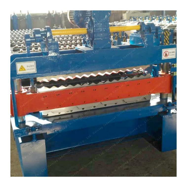
Components of double layer corrugated roof sheet making machine
