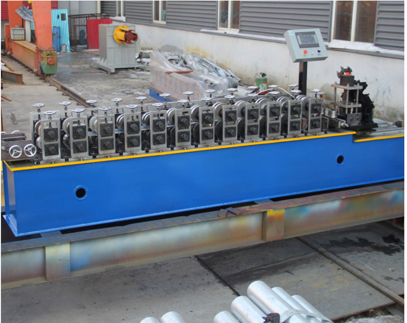
C channel light steel keel roll forming machine picture display
