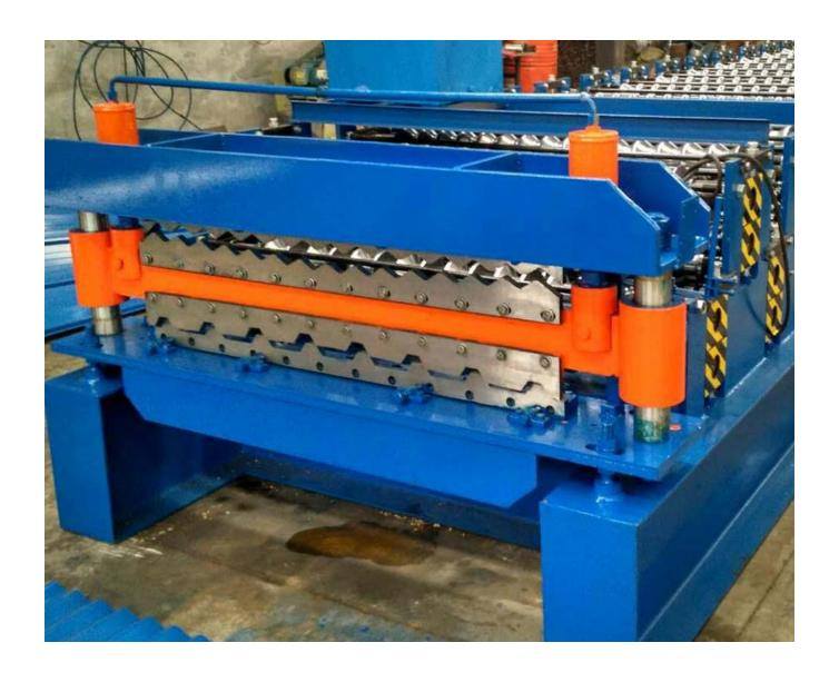
Components of double layer roll forming machine for roof use
