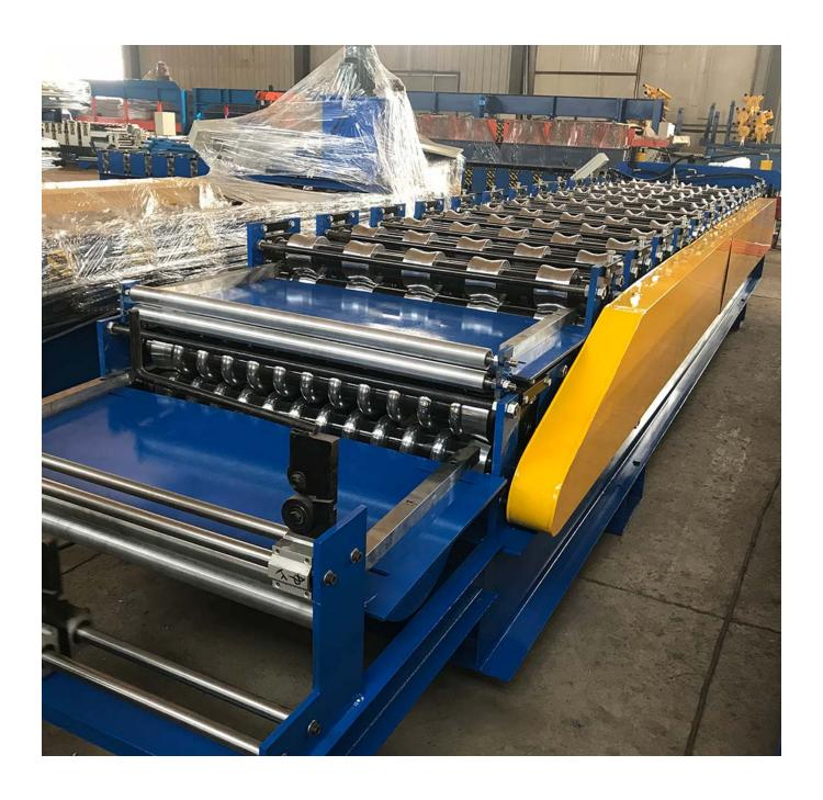
Components of double layer corrugated roof sheet making machine
