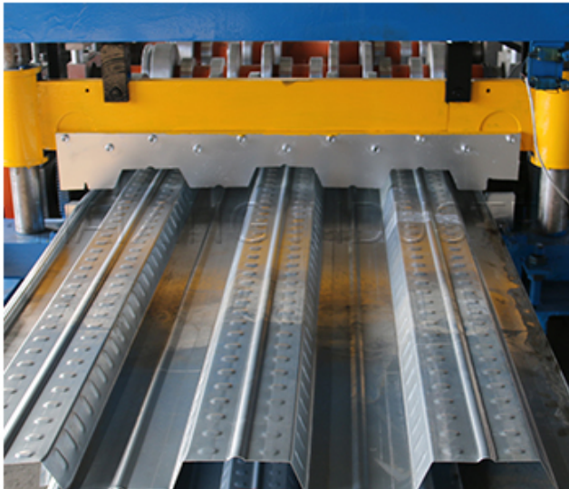
Deck Floor Rolling Production Line details
