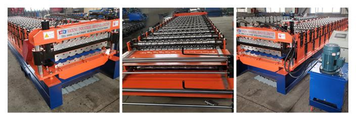
This machine can produce two different types of metal tile products. The upper layer of the machine can form corrugated tiles, and the lower layer of the machine can form trapezoidal tiles. The final product is as follows:
