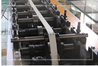
Automatic Ceiling Grid T Bar Sheet Metal Roll Forming Machines' out table uses Stainless operation table, bottom base is welded with iron plate.
