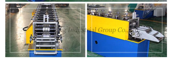
Automatic T Grid Drywall Roll Forming Machine's out table uses Stainless operation table, bottom base is welded with iron plate.
